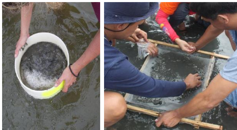
Figure 15. Process of sieving softbottom sediments
